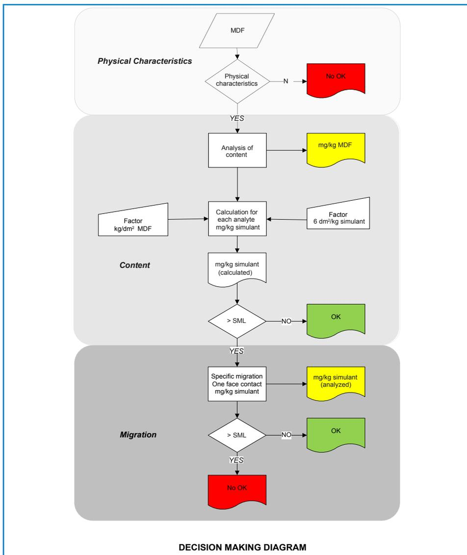
Figure 1. Analytical strategy for conducting migration tests.
