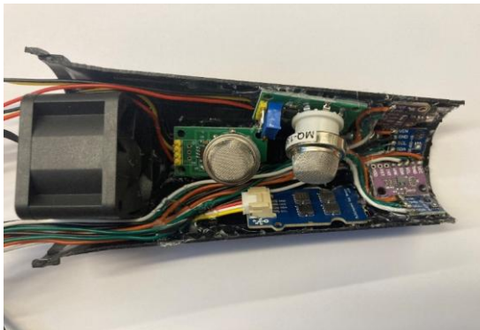
The insides of the electronic nose exposed. 11 different sensors in total.
