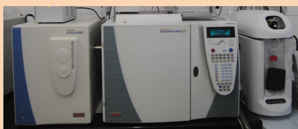
Figure 2: Gas chromatography coupled to mass spectrometry (GC-MS) with purge and trap (P&T) technique
