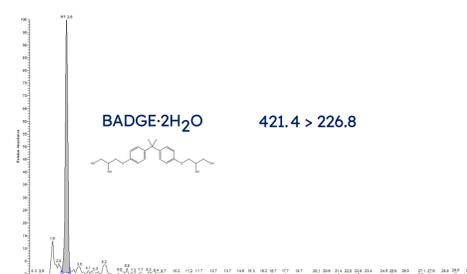
Figure 4. LC-MS/MS chromatogram using negative APCI ionization mode of digested olive oil spiked with BADGE
