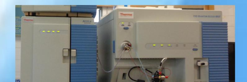
ESI: positive Sheat gas: N<sub>2</sub> Collision Gas: Ar Quantif Trace: DEP (223.1 >149.1), DIBP (279.2 > 149.0), DBP (279.2 > 149.0), BBP (313.1 > 91.1), DEHP(391.3 > 149.0), ATBC (403.2 > 129.0), DEPd(227.2 >153.1)
