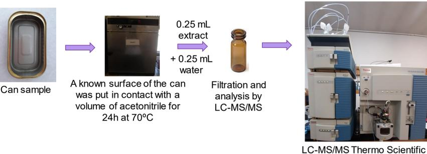
A non-targeted screening by liquid chromatography coupled to tandem mass spectrometry (LC-MS/MS) was performed for migrant identification.
