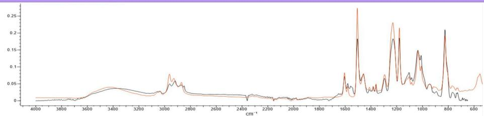
Figure 1. IR spectrum of the internal side of one sample (dark) compared to the IR of the Spectral Library (red)
