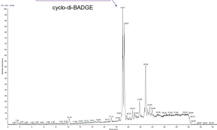
Figure 2: TIC chromatogram for the extract of the beverage sample in positive mode.
