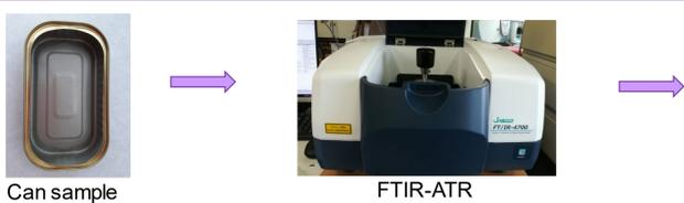
To identify the type of coating, infrared spectra were acquired using an ATR (attenuated total reflectance)-FTIR spectrometer equipped with a diamond optical crystal. The spectra identification was performed by comparing recorded spectra with several commercial spectral libraries (IR Spectral Libraries of Polymers & Related Compounds from Bio-Rad Laboratories).
