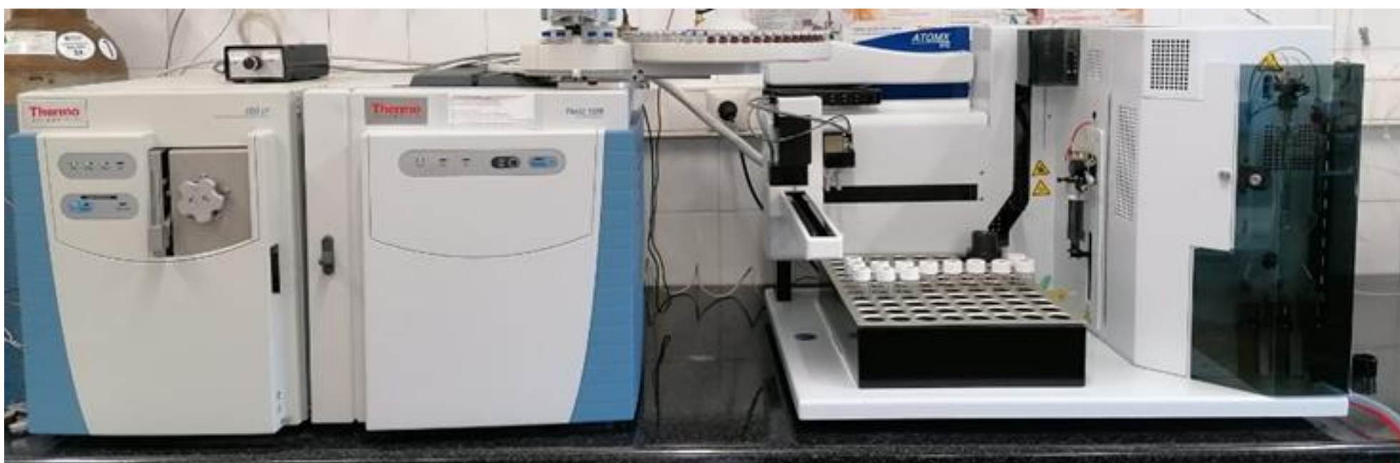
Fig.1.- Purge & Trap system coupled to Gas chromatography-Mass Spectrometry (P&T-GC-MS)
